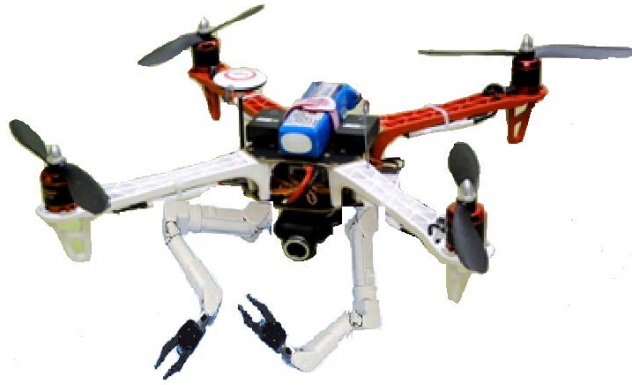
Figure 2.2 Flying Robot with Manipulator (Composite Picture)
